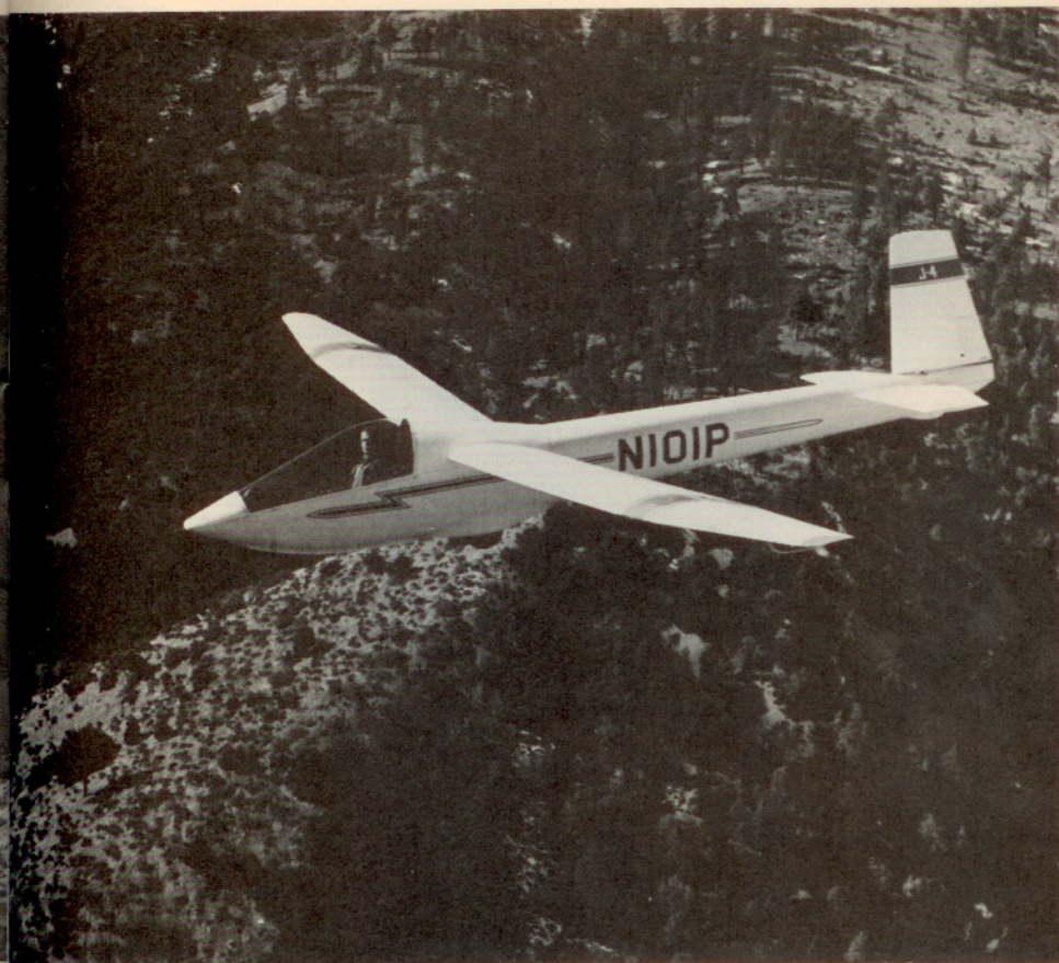
Javelin J-4 near Tehachapi, Calif. Latest 15-meter sailplane has better than 30:1 glide ratio, is now in volume production.
